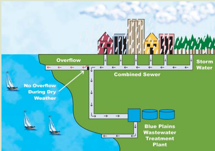
(L) Shows how the District of Columbia's combined sewer system works. (R) Shows WASA's 20 Year Long-Term CSO Control Plan (LTCP) to improve water quality in the Anacostia and Potomac rivers and Rock Creek, the 20-year Long-Term CSO Control Plan includes: three deep underground storage tunnels, including side tunnels to reduce flooding; rehabilitation of existing pumping stations; and the elimination of 14 overflow outfalls. Various sections of this system will be placed in operation along the way to reduce overflows even before the entire project is completed.
