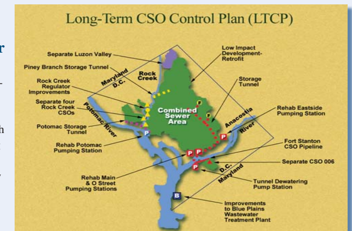
To improve water quality in the Anacostia and Potomac rivers and Rock Creek, the 20-year Long-Term CSO Control Plan includes: three deep underground storage tunnels, including side tunnels to reduce flooding; rehabilitation of existing pumping stations; and the elimination of 14 overflow outfalls. Various sections of this system will be placed in operation along the way to reduce overflows even before the entire project is completed.
