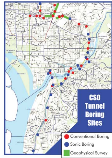
The dots on the map represent locations where soil borings have been taken to determine tunnel routes. Routes under consideration will take the 12- to 23-foot-diameter tunnels beneath the Anacostia River and the Metro subway system.
