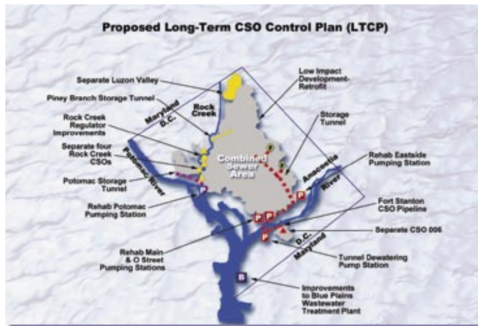
To improve water quality in the Anacostia and Potomac rivers and Rock Creek, the 20-year Long-Term CSO Control Plan includes: three deep underground storage tunnels, including side tunnels to reduce flooded areas; rehabilitation of existing pumping stations; and the elimination of 14 overflow outfalls. Various sections of this system will be placed in operation along the way to reduce overflow pollution even before the entire project is completed.
