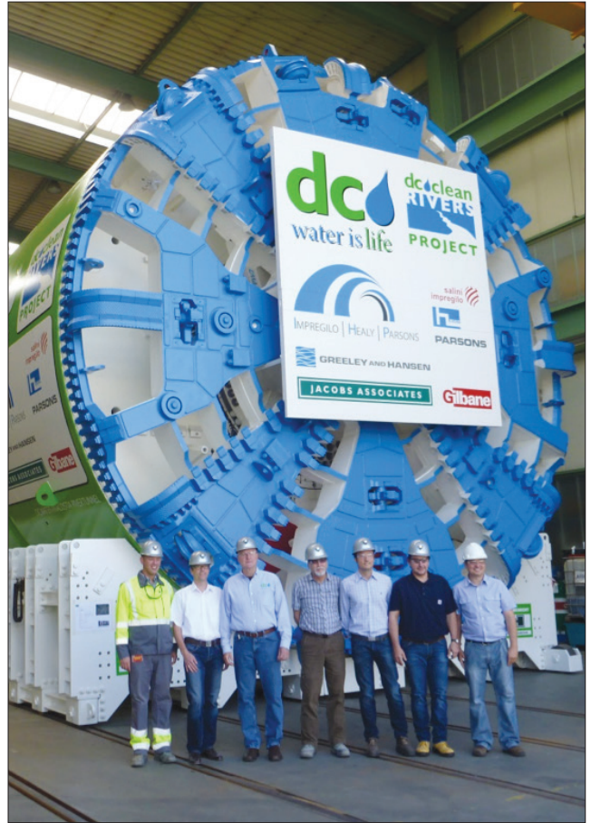
Anacostia River Tunnel Boring Machine
