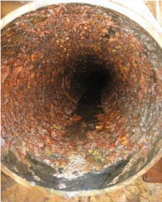
30-inch Tuberculated cast iron pipe (Rhode Island Ave)
