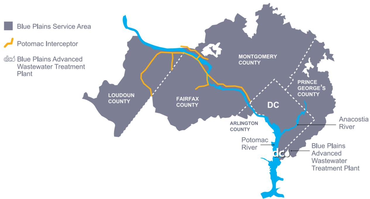
1. DC Water's Blue Plains Advanced Wastewater Treatment Plant is the largest plant of its kind in the world. It has a design average treatment capacity of 384 million gallons per day (MGD), a peak four-hour capacity of 555 MGD, and an additional wet weather treatment capacity of 225 MGD.
