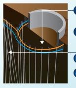
331 four-inch-diameter steel pipes were drilled about 150 feet deep to carry the chilled brine to the specific ground we needed frozen.
