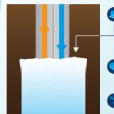
Ice columns between nearly seven and 10 feet thick are formed by each freeze pipe after six to eight weeks of chilled brine being pumped through them. Together, these columns form a structurally sound and watertight ice wall around shafts to be excavated.
