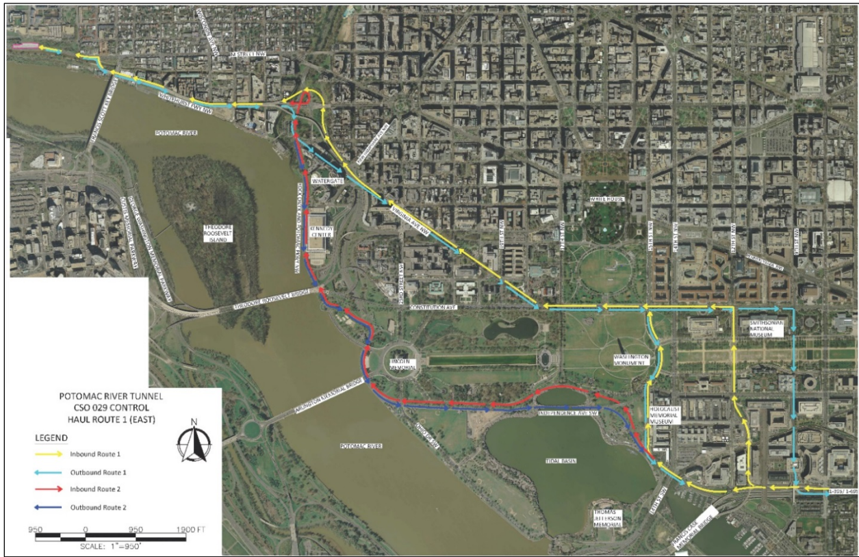
Figure 5: Haul Route 1 (East) for CSO 029 Control
