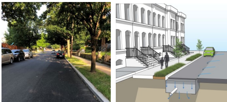
Parking Lane Permeable Pavement (PPP)
