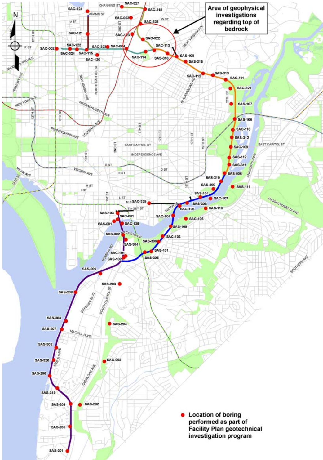
Figure 9: Locations of Borings and Geophysical Survey
